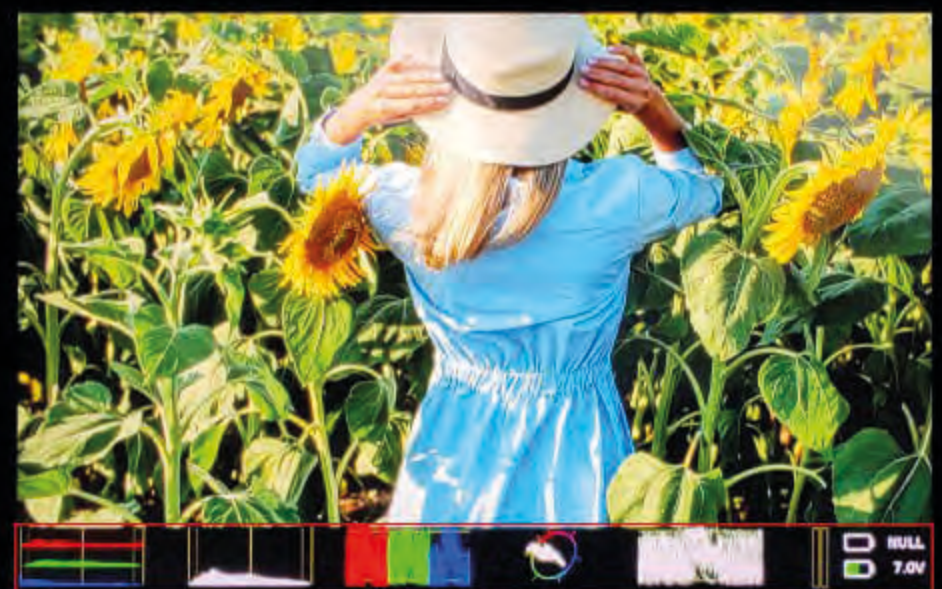
All-waveform( LUM/RGB/VEC Waveform、LUM/RGB Histogram)、Stereo Audio Meters
